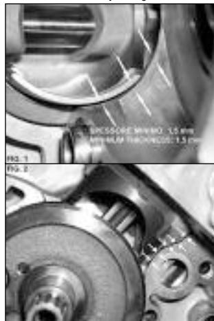
**SQUISH:** To get the best performance from this kit, it is necessary that the squish is equal to 0,9 mm for the kit d. 54. The squish can be measured as follows: move the piston manually at the bottom dead centre. Insert a tin thread of 1,5 mm through the spark plug hole in axis with the piston pin and make the piston turn twice or three times. The tin thread will show a crush that, measured with a centesimal gauge, indicates the squish value (0,9mm).
